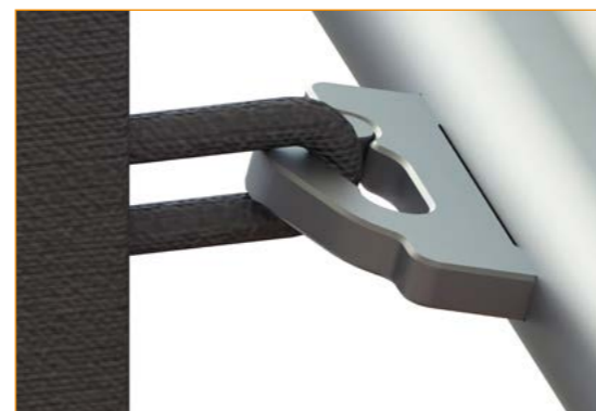
Detail of the hook pressing
